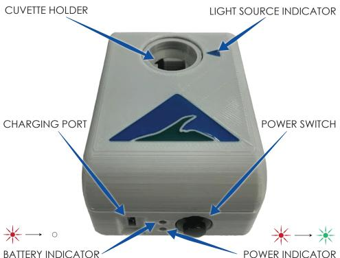
When charging and below 100% battery life, this light will be illuminated red. Light turns off when fully charged.
